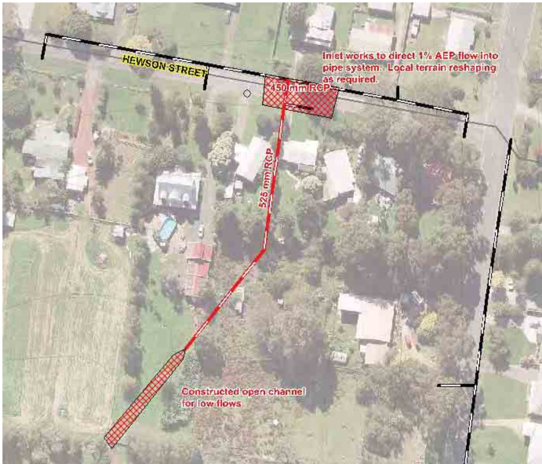
Figure 5.1 Hewson Street flood mitigation works
