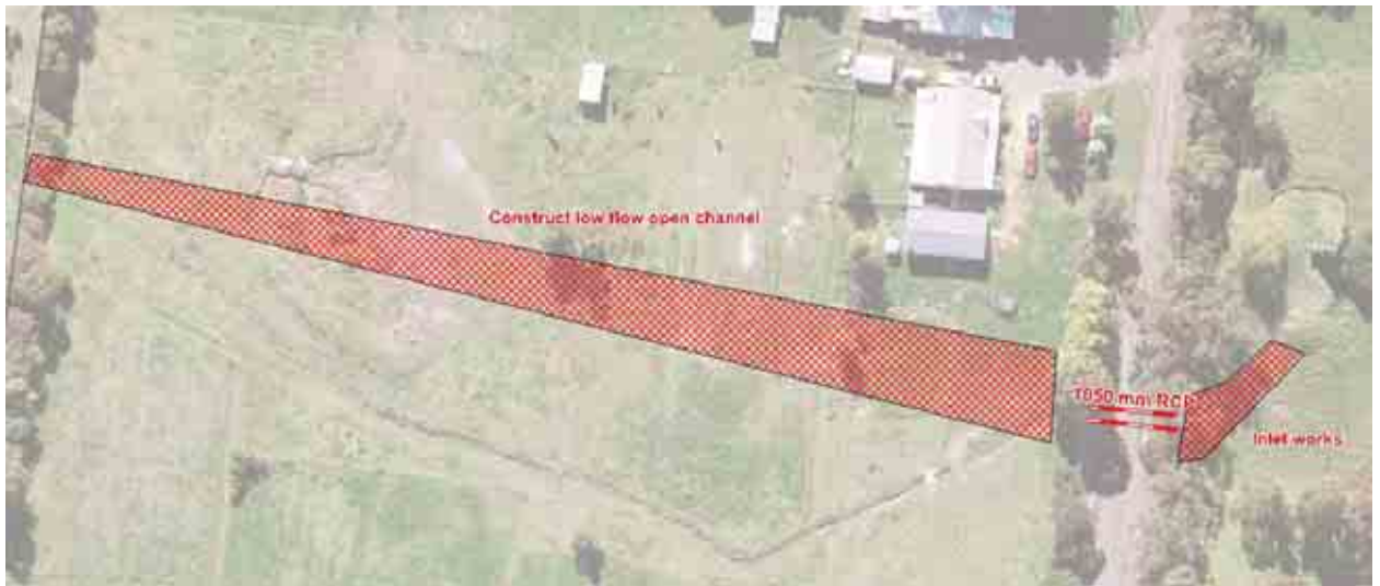
Figure 5.4 Walter Street flood mitigation works
