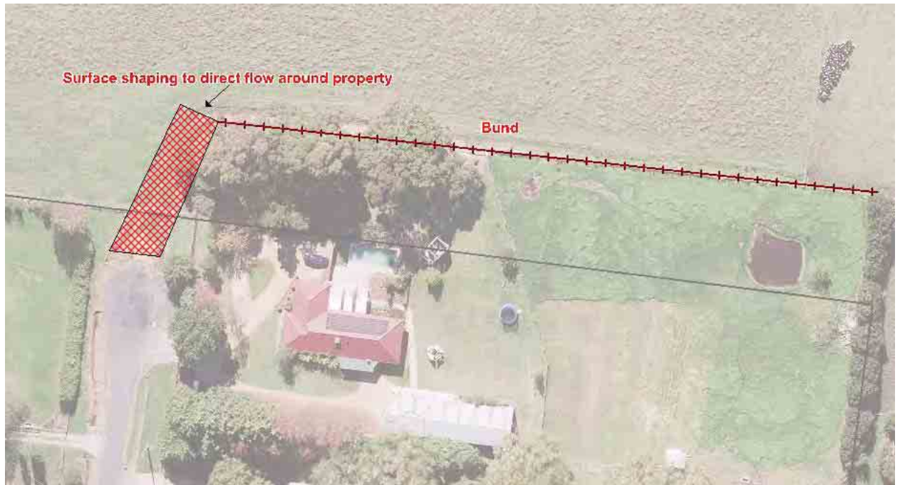
Figure 5.6 Hatches Road flood mitigation works
