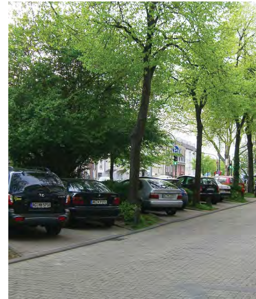
Tree island planting surrounded by kerb and channel is proposed between angled parking spaces (example above).
