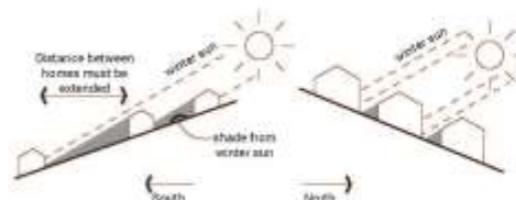
Diagram showing why greater separation is needed between dwellings on south-facing slopes to ensure good solar access is achieved
