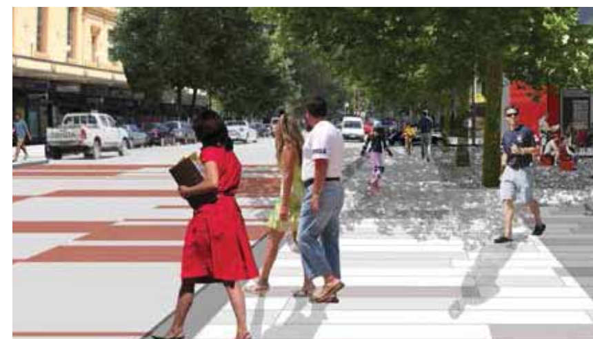
Example: Identify pedestrian priority zone through raising the road table and using contrasting pavement/ surface treatments
