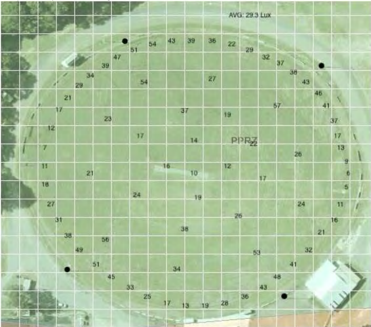
Figure 1 Walter J Tuck Main Oval - Current lux readings indicate an average of 29.3 Data provided by Ace Earthmoving P/L
