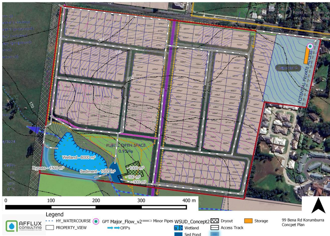
Figure 60. Indicative Drainage Concept Plan - Waterway Realignment
