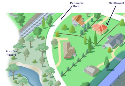
Illustration of a perimeter road at the edge of a settlement (Figure 6 from [DELWP 2020 Design Guidelines for Settlement Planning at the Bushfire Interface](#))
