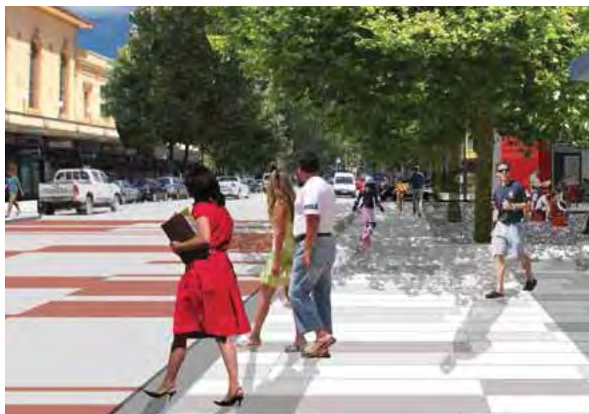
Example: Identify pedestrian priority zone through raising the road table and using contrasting pavement/ surface treatments
