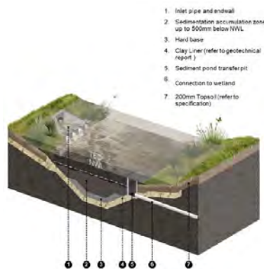
Figure 14: Typical Sediment Basin Profile
