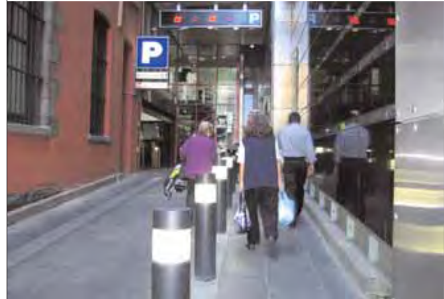
AVOID PLACING BOLLARDS WITH INTEGRATED LIGHTING CLOSE TO PATHWAYS AS IT CAN CAUSE A BLINDING EFFECT FOR PEDESTRIANS AND CYCLISTS.
